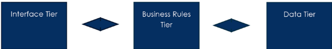
Figure 2-5. Three-tier modular application design
