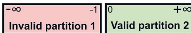
Figure 2-5. The equivalence classes of the input parameter for the number of days
